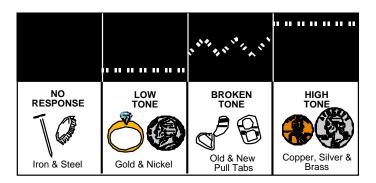
Adjust the DISCRIMINATE control higher to increase the range of the low tone. It is possible to set the DISCRIMINATE level so that nickels have a low tone, larger coins have a high tone and pull tabs have an in-between "broken" tone, making them easily recognizable.
