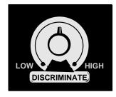
Sensitivity will be slightly reduced when using either the DISC or TONE Discriminator.
