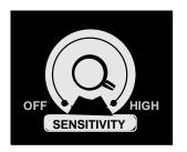
For maximum performance, operate with the sensitivity as high as possible. The sensitivity can generally be set higher when the Discriminator is on.
